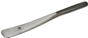
**Spoons -** spoons are used for bumping and prying, they can also be used instead of a dolly when direct access to the rear of a panel is obstructed. The choice of spoon depends on the original contour of the metal, the amount of access available and the proposed action (ie roughing or levelling).
