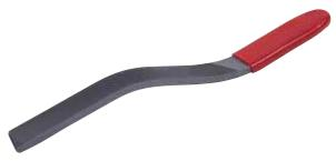
**Bumping Tools** - these are used for slapping out dents, with or without the backing support of a dolly. (For slight dents or a wavy surface, a dolly is not required). They should only be used where damage is moderate or slight, they are not intended to take the role of the spoon or beater and dolly.
